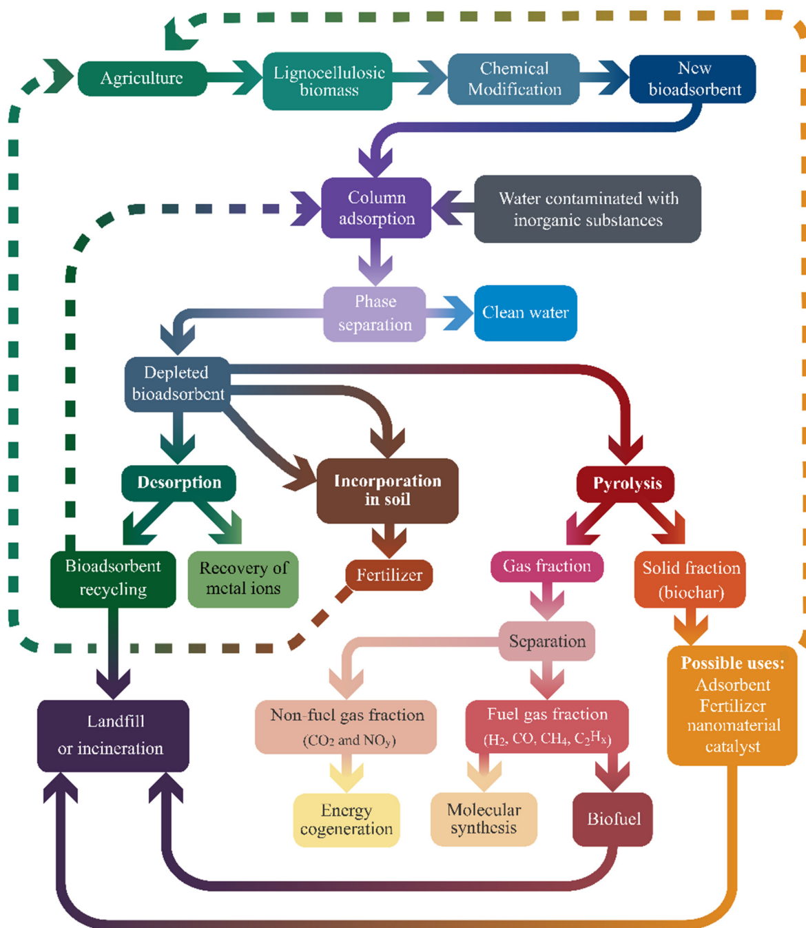
Figure 11. Flowchart for use and destination of lignocellulosic adsorbents. Adapted from Badescu et al. [181].
