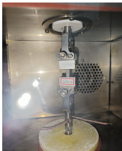
Figure 2. Connection method between the fixture and DMA.
