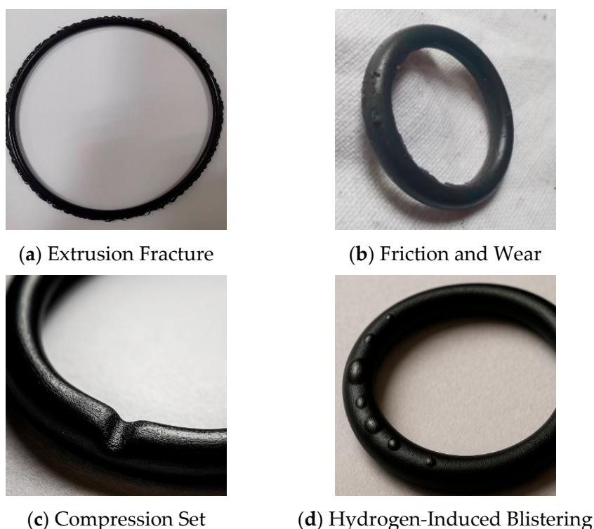
Figure 2. Common failure modes of O-rings in high-pressure hydrogen environments.
