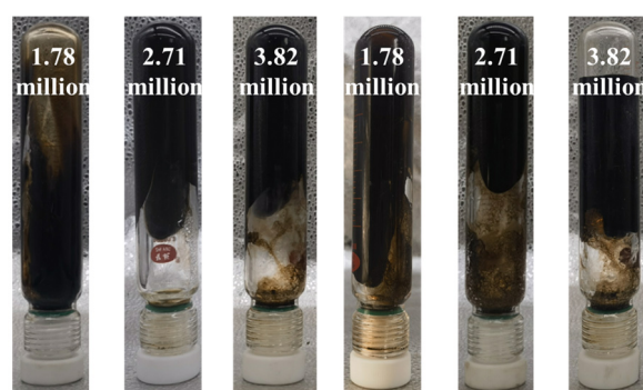
Figure 6. Gelation behavior of polymers with different molecular weights ((left): after aging 8 h; (right): after aging 6 h).
