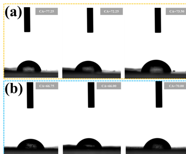
Figure 7. Water contact angle image of (a) pure PLA; (b) 1%CNWs-0.5%Nano-TiO 2 /PLA composite film.
