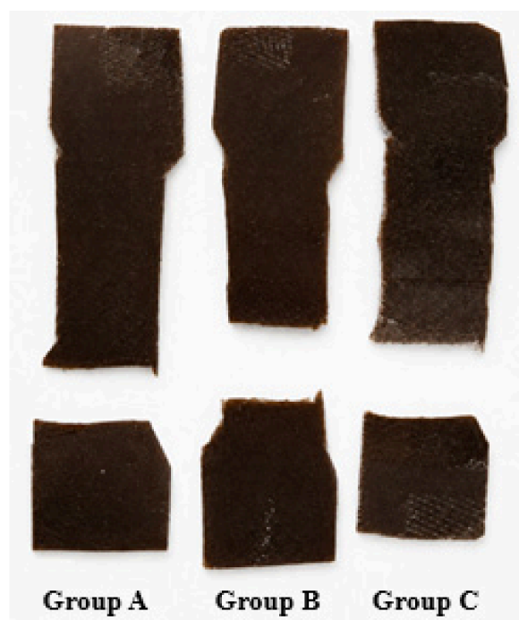
Figure 3. Photographs of tensile-fractured composite specimens after tensile testing. Groups A, B, and C represent epoxy composites containing 1, 3, and 5 wt.% kraft lignin, respectively, together with a fixed Fe–Mn–Si alloy particle content of 3 wt.%.
