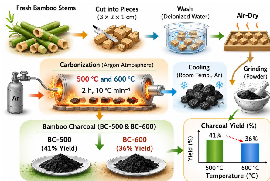
Figure 7. Schematic illustration of the preparation of bamboo charcoal through cutting, washing, drying, carbonization, cooling, and grinding.
