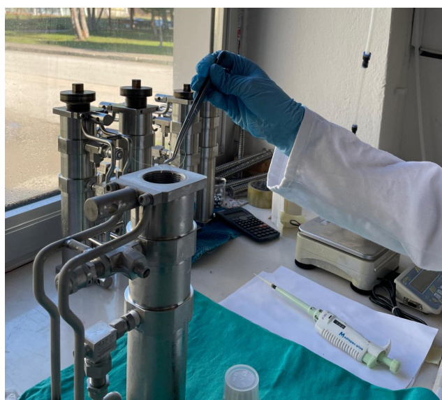
Figure 1. The supercritical carbon dioxide (scCO 2 ) impregnation system used for the incorporation of carvacrol and benzydamine HCl into absorbable surgical sutures.
