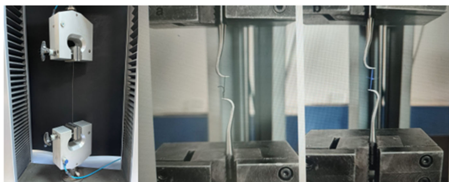
Figure 2. Tensile strength evaluation of untreated, supercritical CO 2 -treated, conventionally impregnated, and carvacrol- or benzydamine HCl-loaded absorbable surgical sutures.
