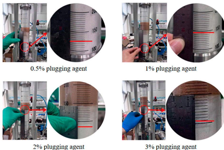
Figure 5. Infiltration depth of sand beds with different concentrations of XZ.
