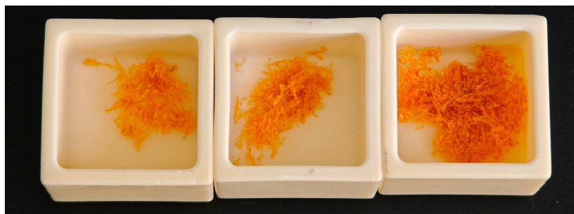
Figure 6. Crosslinked product of TPU after UV aging.
