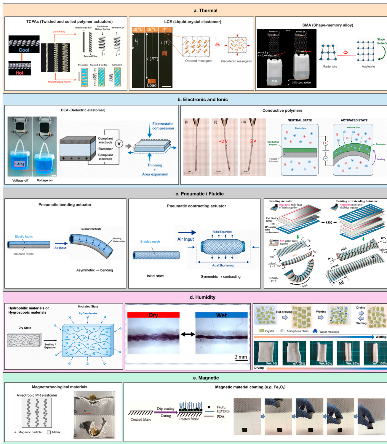
Figure 2. Material classification, actuation mechanisms, and structural motion modes of active fibers and fabrics categorized by driving stimuli. (a) Thermal actuation: Twisted and coiled polymer actuators (TCPAs) generating contraction through anisotropic thermal expansion and helical unwinding, which is different from simple helical structure (adapted with permission from ref. [34], copyright 2014, AAAS; and ref. [35] under the Creative Commons CC BY license); liquid-crystal elastomers (LCEs) undergoing reversible axial contraction triggered by order-disorder mesogen phase transitions upon heating (adapted with permission from ref. [77], copyright 2021, AAAS); shape-memory alloys (SMAs) recovering memorized shapes via temperature-induced martensite-to-austenite phase transformation (adapted with permission from ref. [33], copyright 2026, AAAS). (b) Electrical and Ionic actuation: Dielectric elastomer actuators (DEAs) operating via electrostatic Maxwell stress-induced
