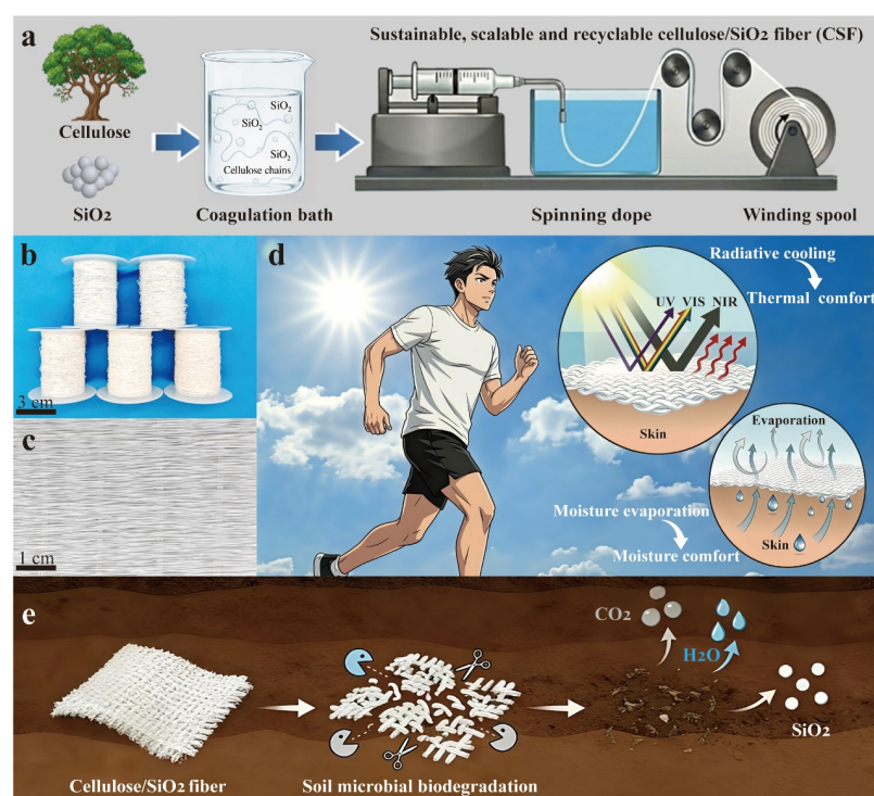
Figure 1. Preparation of sustainable and scalable cellulose/ \text{SiO}_2 fiber. (a) A schematic illustration of the green wet-spinning process for preparing CSF, including the cellulose/ \text{SiO}_2 precursor system, spinning-dope preparation, fiber regeneration in the coagulation bath, and continuous winding. (b) A photograph of the continuously collected CSF. (c) A photograph of the CSF woven into the textile. (d) A schematic illustration of the mechanism of thermal and moisture comfort of CSF, showing radiative cooling through solar reflection and mid-infrared heat emission, together with moisture evaporation enabled by sweat evaporation at the skin–CSF interface. (e) An illustration of the end-of-life biodegradation pathway of the CSF in soil, where the cellulose component undergoes soil microbial biodegradation accompanied by the release of \text{CO}_2 and \text{H}_2\text{O} , while nano- \text{SiO}_2 is returned to the natural environment as an environmentally benign inorganic component.
