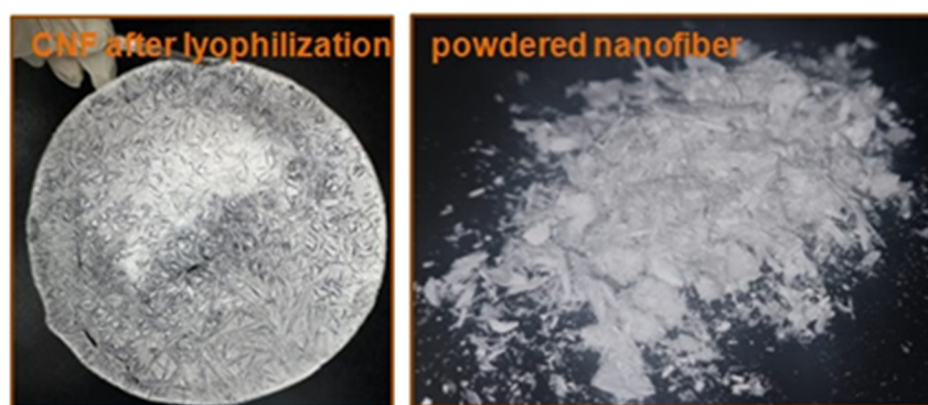
Figure 3. CNF obtained from MCC.
