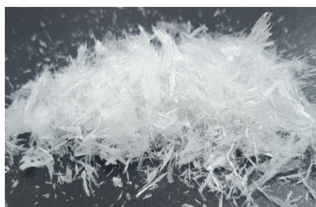
Figure 4. CNC obtained from MCC.
