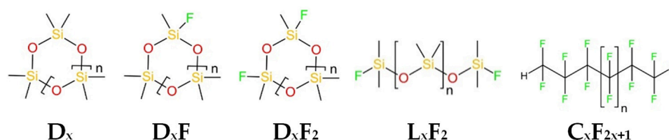
Figure 4. Proposed major liquid product groups formed during PTFE:SR co-pyrolysis based on GC–MS and NMR analysis. Structural assignments are tentative and were derived primarily from mass spectral interpretation.
