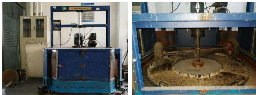
Figure 3. Accelerated abrasion test apparatus for road marking paints.
