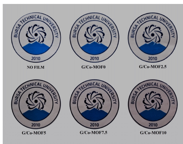
Figure 3. Visual appearances of G/Co-MOF composite films. G/Co-MOF0: Gelatin film without cobalt metal–organic framework; G/Co-MOF2.5: Gelatin film with 2.5% cobalt metal–organic framework; G/Co-MOF5: Gelatin film with 5% cobalt metal–organic framework; G/Co-MOF7.5:
