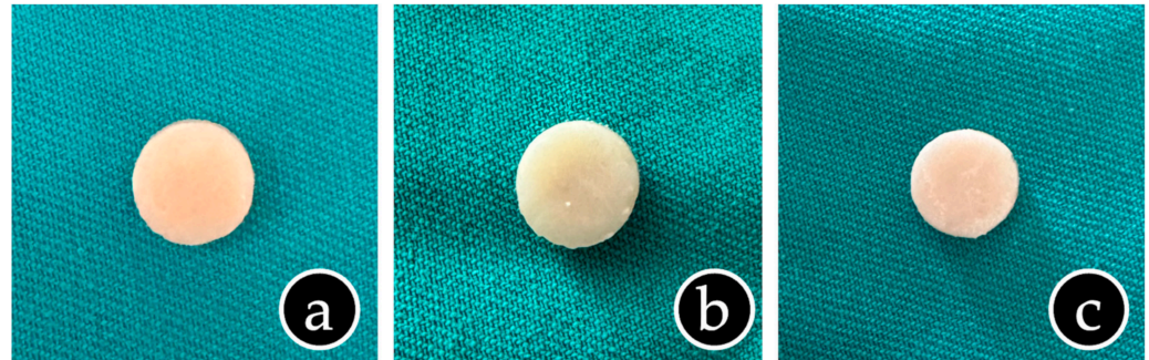
Figure 1. Representative disc-shaped specimens prepared from the three restorative materials evaluated in the study: (a) compomer (Dyract XP); (b) microfilled hybrid composite resin (G-aenial Posterior); and (c) glass hybrid restorative system (EQUIA Forte HT).
