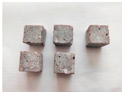
Figure 1. The UPC specimens used for the water absorption test.
