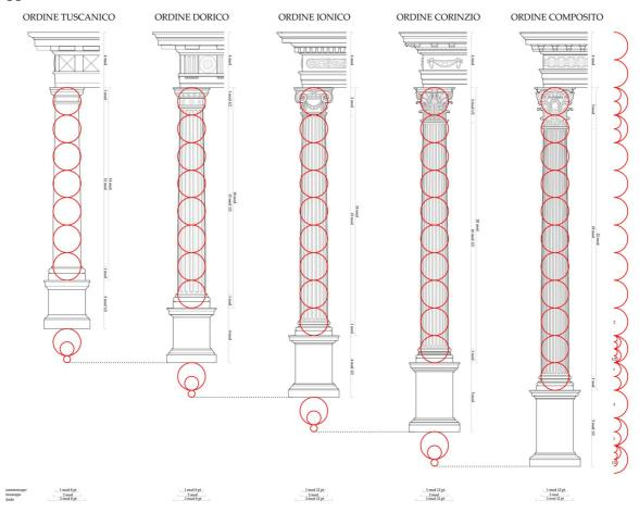
**Figure A1.** Drawing of the comparison between the architectural orders with the analysis of the reduction ration.
