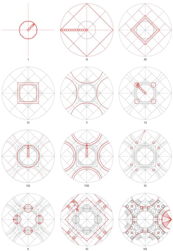
**Figure A2.** Geometrical proportional scheme to create the plan de-composed in 12 essential passages: starting from the central octagon, the wall cell, the position of columns in the peristyle, the limit of the base, the openings and stairway are defined.
