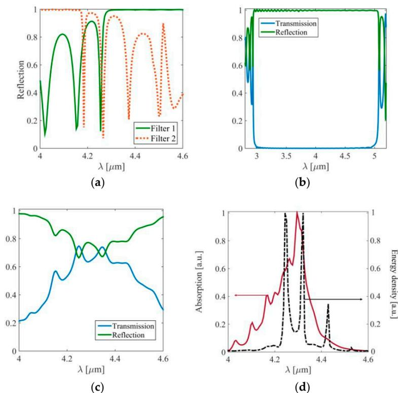
**Figure 2.** Optical response of the individual sections of the structure: (a) Filters 1 and 2; (b) Mirror; (c) Matching section; (d) Response of the whole structure for an excitation of the fundamental slab mode in the slab region; Red thick line corresponds to the absorption of the system when filter 1 is undoped and black dashed line shows the energy density when all components are undoped.
