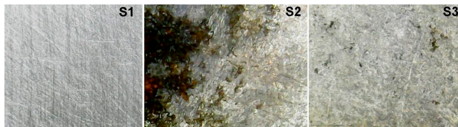
Figure 2. Surface morphology images of the carbon steel: blank (S1); immersed in seawater without natural seaweeds (S2); immersed in seawater with natural seaweeds (S3).
