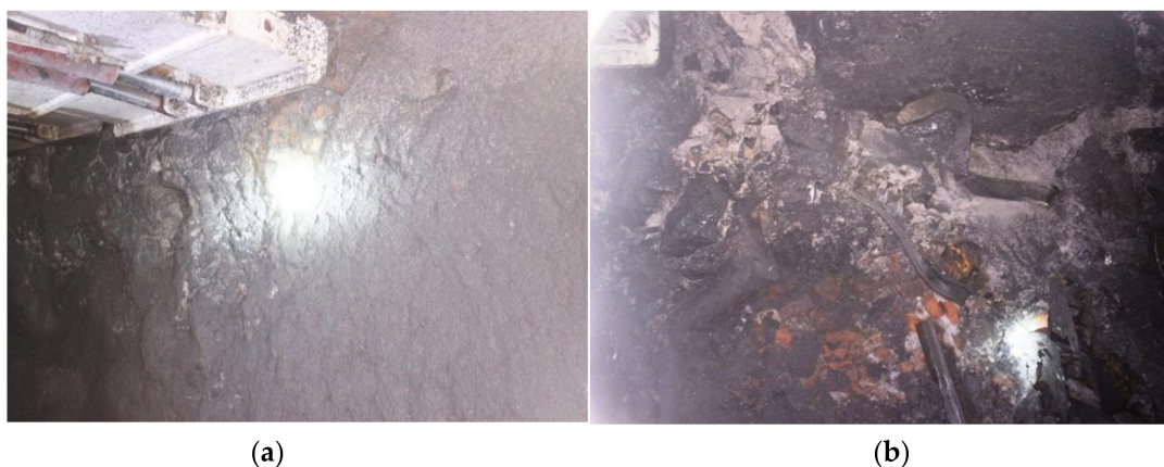
Figure 16. The rock mass exposed in the grouting area: (a) Coal wall; (b) Tip-to-face roof.
