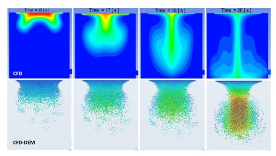
**Figure 10.** A comparison of the CFD and CFD–DEM results for matte settling in the small-scale settler model, revealing a similar funneling flow pattern at 15, 17, 18, and 20 s. Upper row: CFD, lower row: CFD–DEM.
