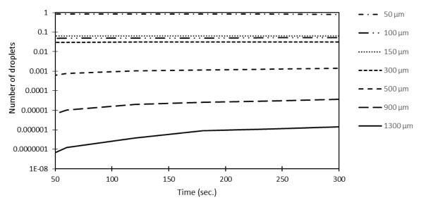
Figure 4. Number fraction distribution of different-sized droplets inside the settler.
