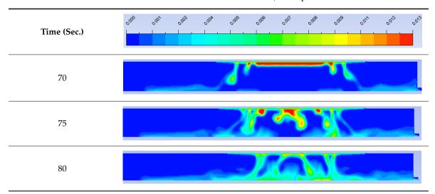
Table 6. Volume fraction contours for 500 μm droplets.
