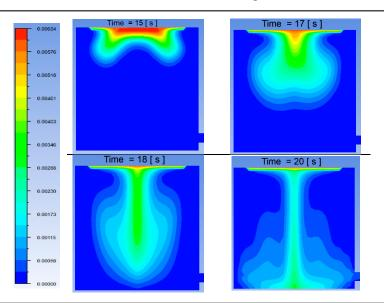
Table 4. Volume Fraction Contours for 500  $\mu$ m Droplets at 15, 17, 18, and 20 s.
