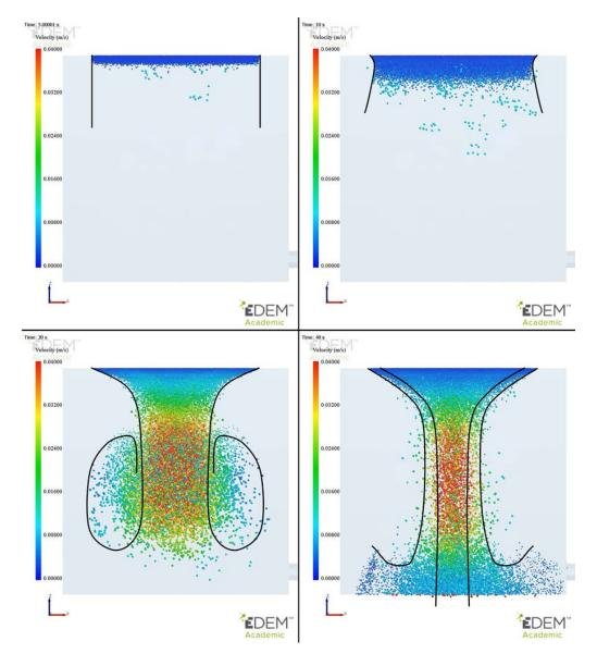
Figure 6. Formation of the funneling effect in the slag at 5 s, 10 s, 20 s, and 40 s.
