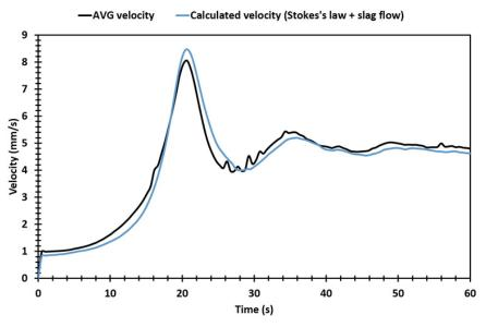
Figure 7. Average velocity of droplets and calculated velocity.
