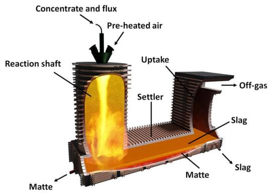
Figure 1. Illustration of the Outotec flash smelting furnace.
