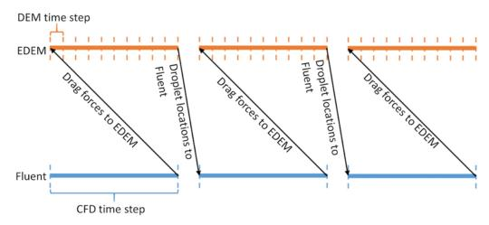
**Figure 2.** Illustration of the computational fluid dynamics–discrete element method (CFD–DEM) calculation process.
