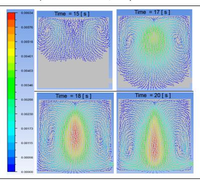
Table 5. Velocity Vector Contours for 500  $\mu$ m Droplets at 15, 17, 18, and 20 s.
