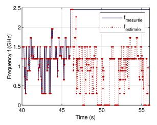
**Figure 14.** Estimated frequency from loads against measured frequency that is blocked at the maximum value around t = 46 s.
