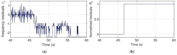
**Figure 15.** Profile of the frequency residuals during faulty operation. Frequency is blocked at the maximum value around t = 46 s at which time an alarm is generated. (a) Raw residuals  $r_f$ . (b) Averaged residuals  $R_f$ .
