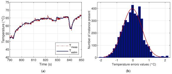
**Figure 10.** The Autoregressive–Moving-Average with Exogenous Inputs (ARMAX) temperature model perfomance. (a) ARMAX model temperature estimations compared to system readings. (b) Distribution of the ARMAX Temperature estimation errors.
