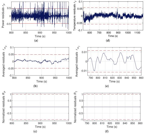
**Figure 13.** Power and temperature residuals assessment in normal operation. (a) Power raw residuals  $r_P$ . (b) Power averaged residuals  $r_{m_P}$ . (c) Power normalized residuals  $R_P$ . (d) Temperature raw residuals  $r_T$ . (e) Temperature averaged residuals  $r_{m_T}$ . (f) Temperature normalized residuals  $R_T$ .
