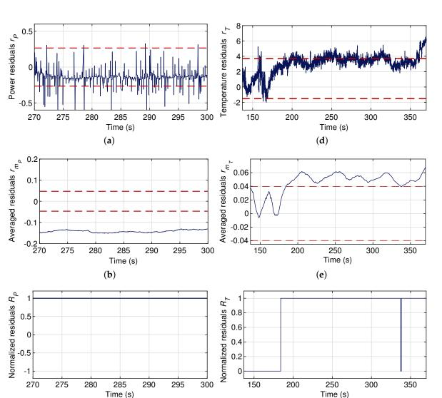
(c) (f) **Figure 18.** Power residuals assessment during faulty scenario of the introduction of an external component, and temperature residuals during the heating experiment. (a) Power raw residuals  $r_P$ . (b) Power averaged residuals  $r_{m_P}$ . (c) Power normalized residuals  $R_P$ . (d) Temperature raw residuals  $r_T$ . (e) Temperature averaged residuals  $r_{m_T}$ . (f) Temperature normalized residuals  $R_T$ .
