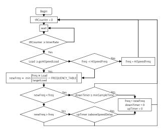
Figure 5. A simplified flowchart for modeling of the Interactive Governor.
