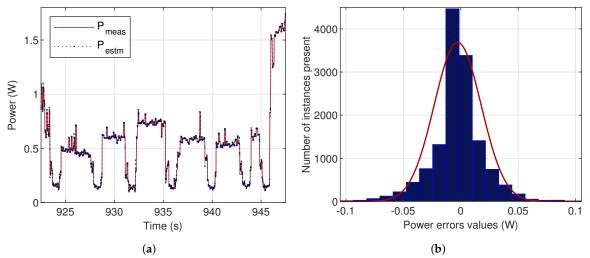
**Figure 9.** NARX power model perfomance. (a) NARX model power estimations compared to the system measurements. (b) Distribution of the NARX power model estimation errors.
