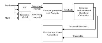
Figure 3. Overview of the proposed monitoring method.
