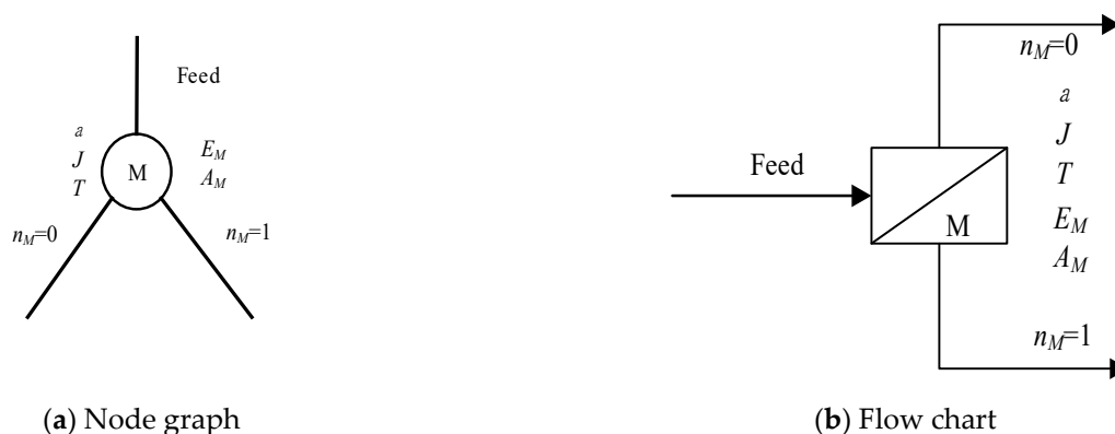
Figure 2. Membrane node graph (a) and membrane module flow chart (b) obtained by decoding.
