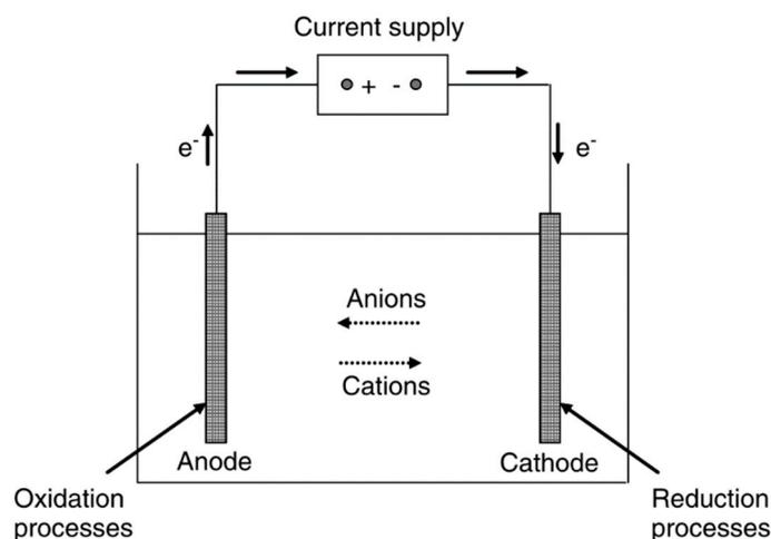
**Figure 2.** Schematic diagram of electrochemical reactor (Adapted from [25]).
