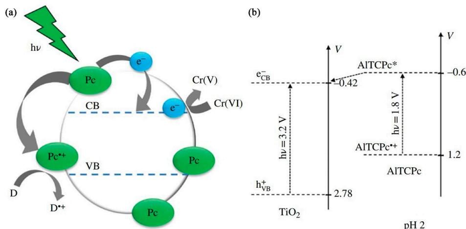
**Figure 3.** (a) Schematic diagram of heterogeneous photocatalytic reduction of Cr(VI) under visible light and (b) energy band of TiO<sub>2</sub> modified with AITCPC (Adapted from [79]).
