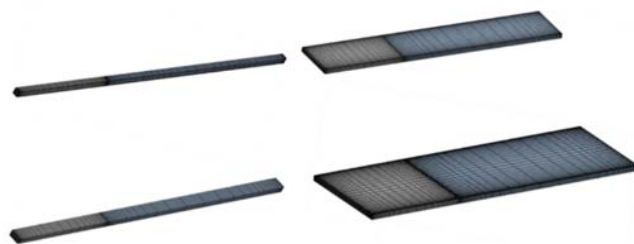
Figure 2. Examples of meshes for 3D geometries with aspect ratios: (top left): 1:1; (bottom left) 2:1; (top right) 10:1; (bottom right) 20:1; In the present work top right.
