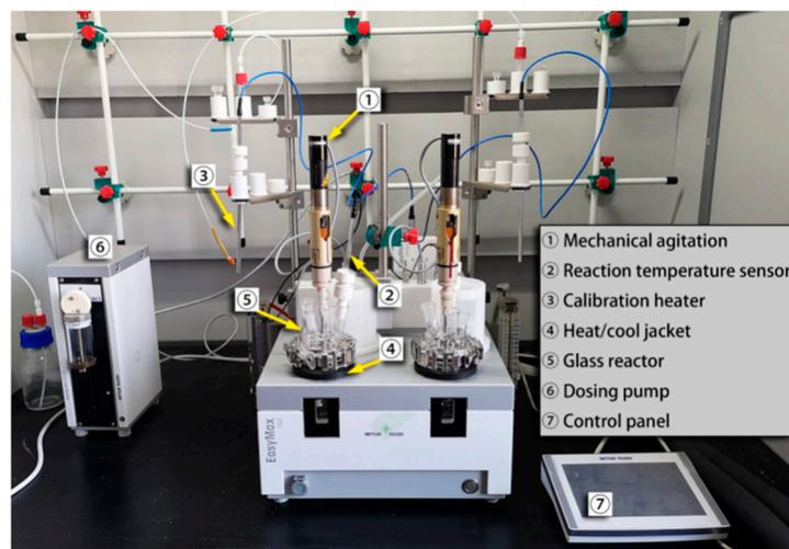
**Figure 8.** The instruments used in the temperature control experiments (EasyMax 102).
