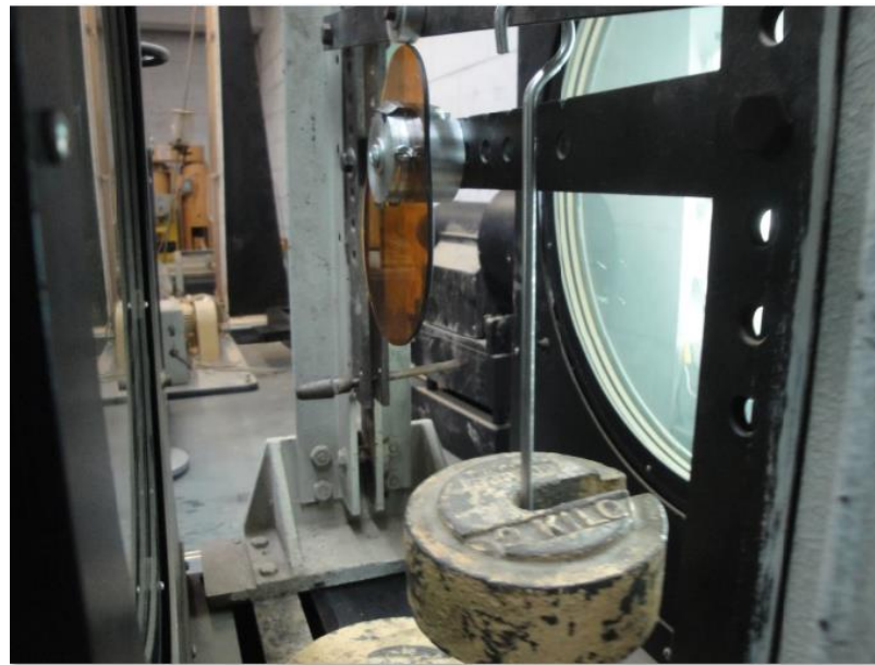
Figure 10. Cam installation on the shaft through square grooving key.
