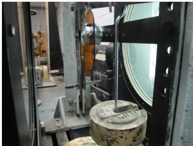
Figure 10. Cam installation on the shaft through square grooving key.
