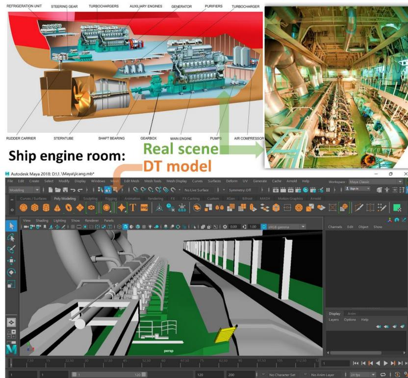
Figure 3. DT modeling for ship engine room.
