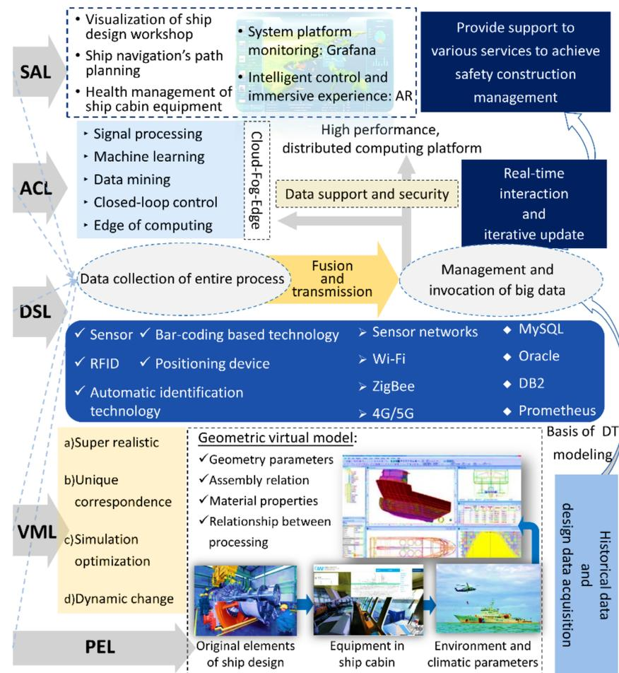
Figure 2. Five-tier framework of process management based on DT-enabled system.
