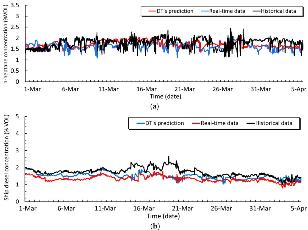
**Figure 8.** Comparison of concentrations with DT's prediction, real-time data and historical data. (a) Time-varying characteristic of n-heptane concentration. (b) Time-varying characteristic of ship diesel concentration.
