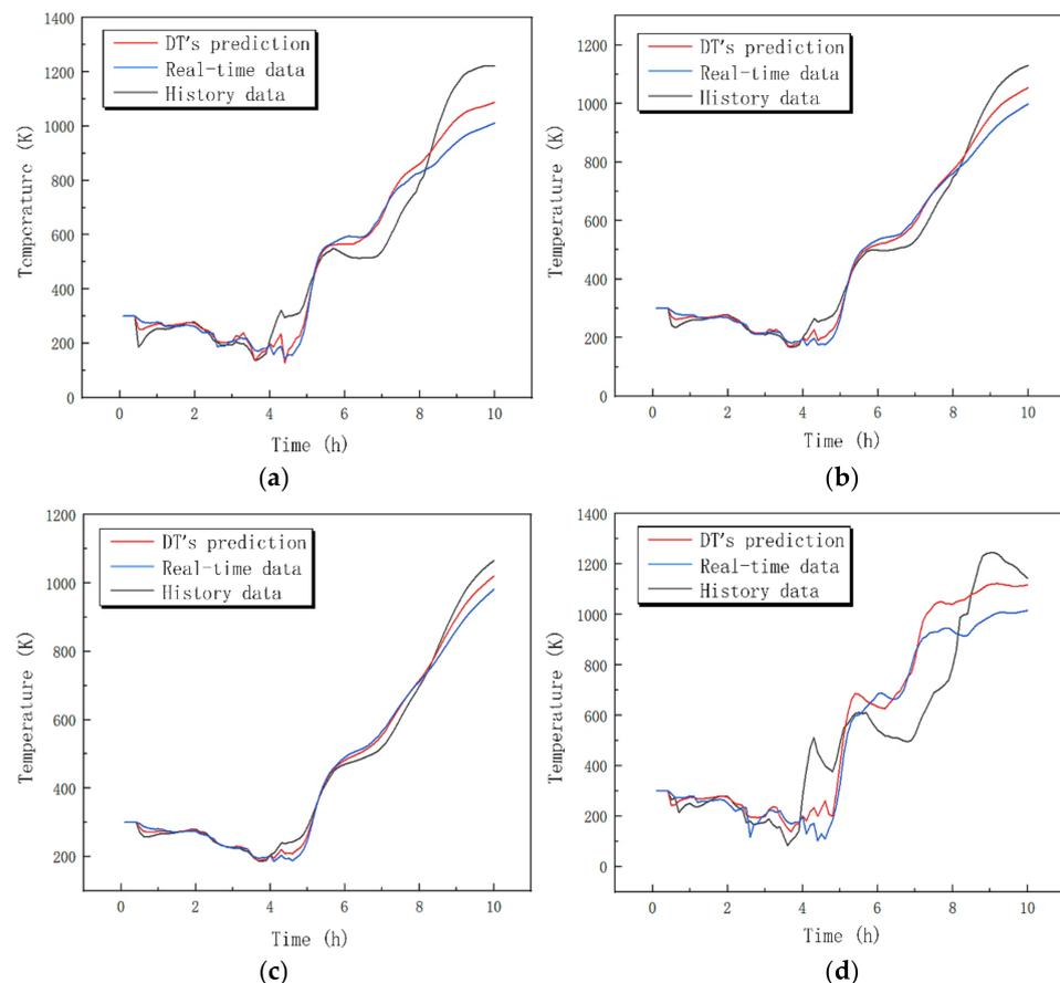
**Figure 5.** Comparison between DT's prediction, real-time data and historical data. (a) Condition 1. (b) Condition 2. (c) Condition 3. (d) Condition 4.
