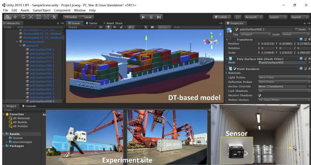
Figure 6. Integrated ship and cargo container with DT modeling combining multilayers.
