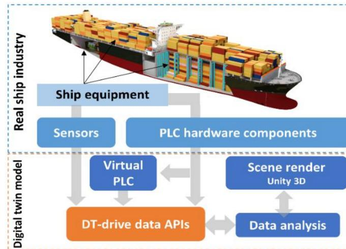
Figure 1. Specific process of data communication between the real scene and DT model.
