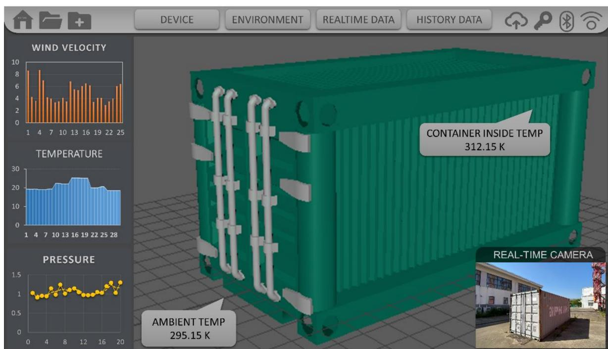
Figure 7. DT-driven platform for shipping cargo container in the operation process.
