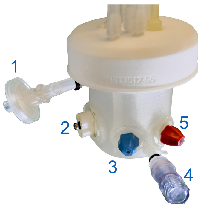
Figure 5. Fully assembled bioreactor. Visible are the baffle aeration connection (1), biomass sensor (2), DO sensor (3), sampling port (4) and the pH sensor (5).
