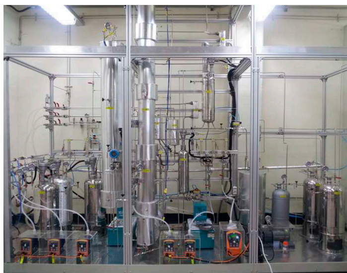
Figure 2. PFR system with the same dimensions used in simulation.
