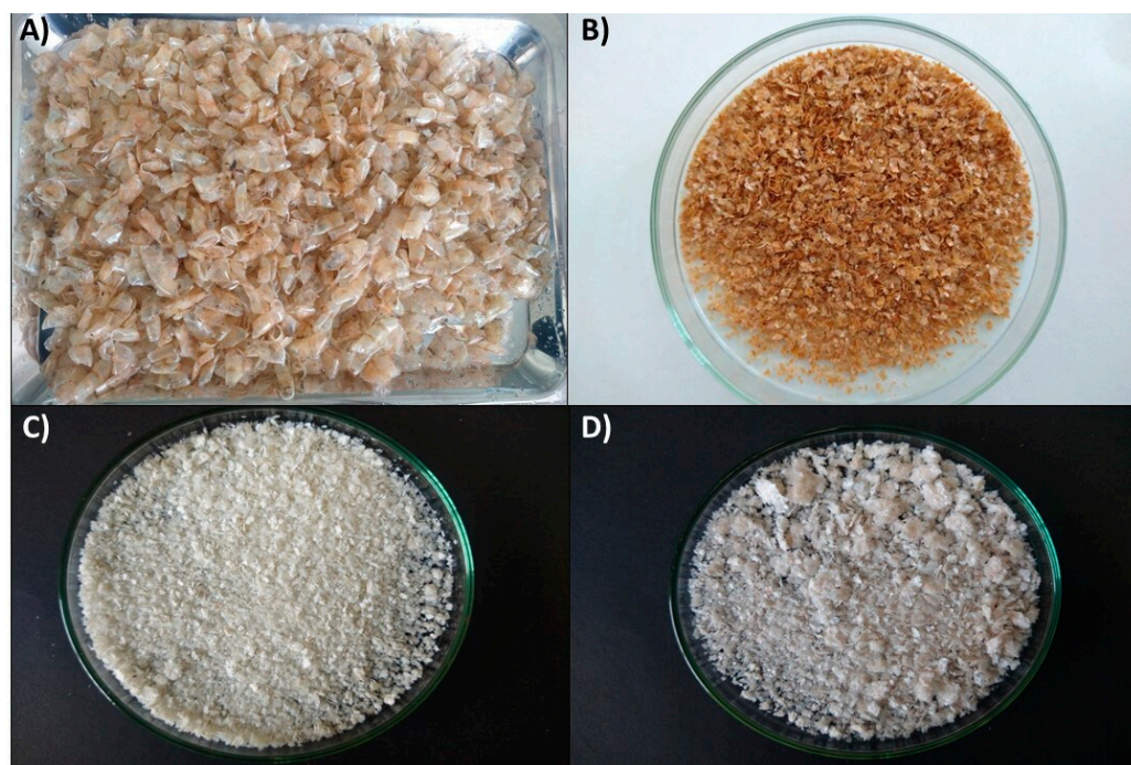
Figure 2. Images of shrimp exoskeleton samples at different stages of chitin extraction: (A) the initial exoskeleton; (B) the conditioned exoskeleton; (C) treatment with Pseudomonas aeruginosa QF50; and (D) treatment with Serratia marcescens QCS23.
