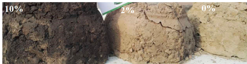
Figure 5. Soil appearance after treatment with different bio-humate acid amendments (10%, 2%, 0%).
