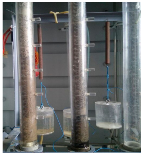
Figure 2. Experimental instrument for the height meter for capillary water rise.
