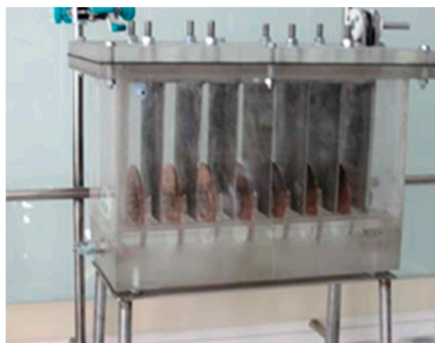
Figure 3. The electrolyzer used for gallium reduction.
