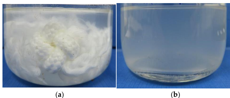
Figure 3. Image of temporary-plugging-knot dissolution. (a) Image of a temporary-plugging knot soaked in water at 60 °C (0 h). (b) Image of a temporary-plugging knot soaked in water at 60 °C (120 h).
