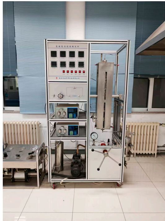
Figure 2. High-temperature and high-pressure foam stability tester.
