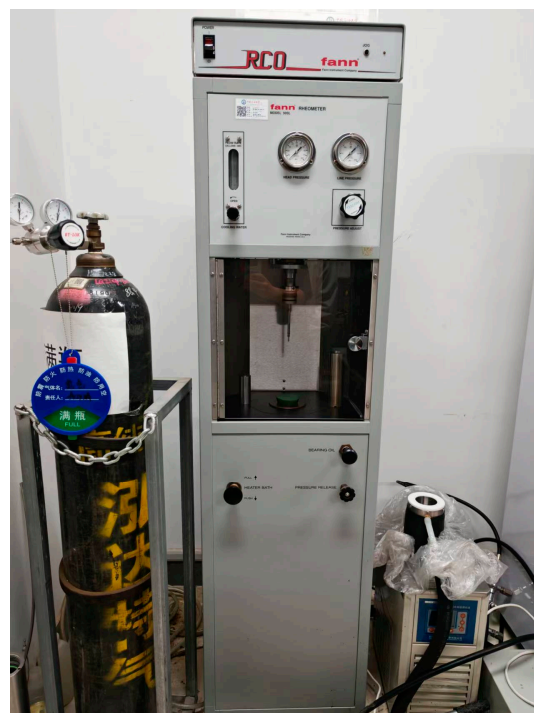
Figure 3. High-temperature and high-pressure rheometer.
