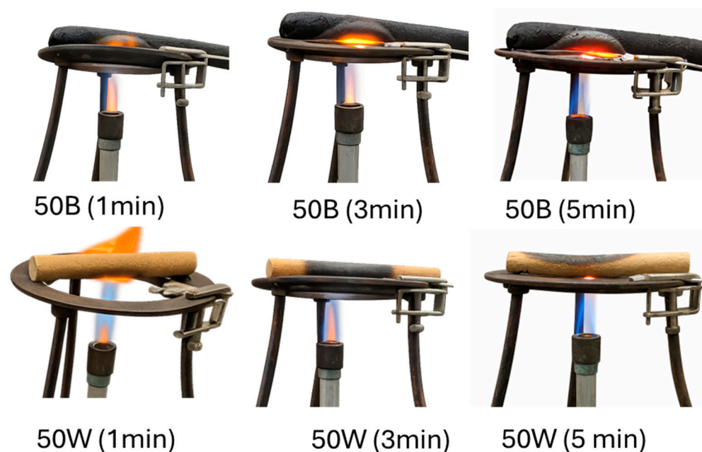
Figure 10. Photographs of the Bunsen burner flame test of the 50B and 50W composites at 1, 3, and 5 min.
