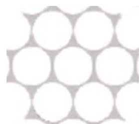
Figure 8. Close-packed pore arrangement in the microfluidic model.
