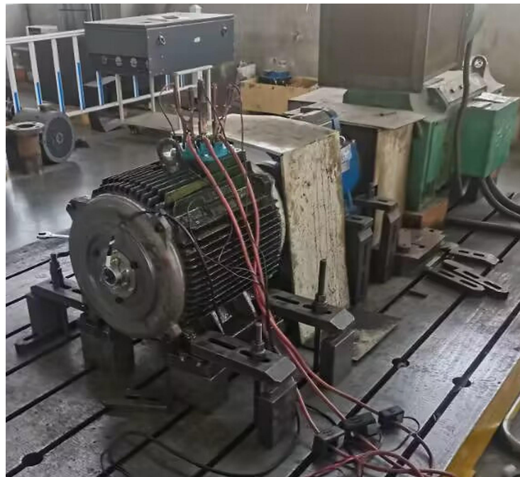
Figure 2. Experimental platform of the synchronous reluctance motor test bench.
