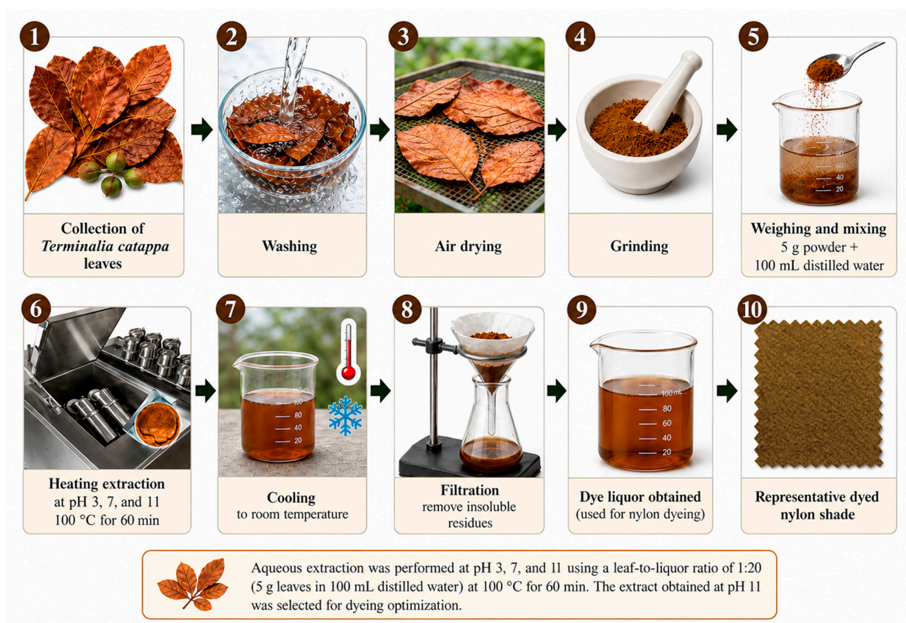
Figure 1. Schematic workflow of mordant-free nylon dyeing with Terminalia catappa leaf extraction.
