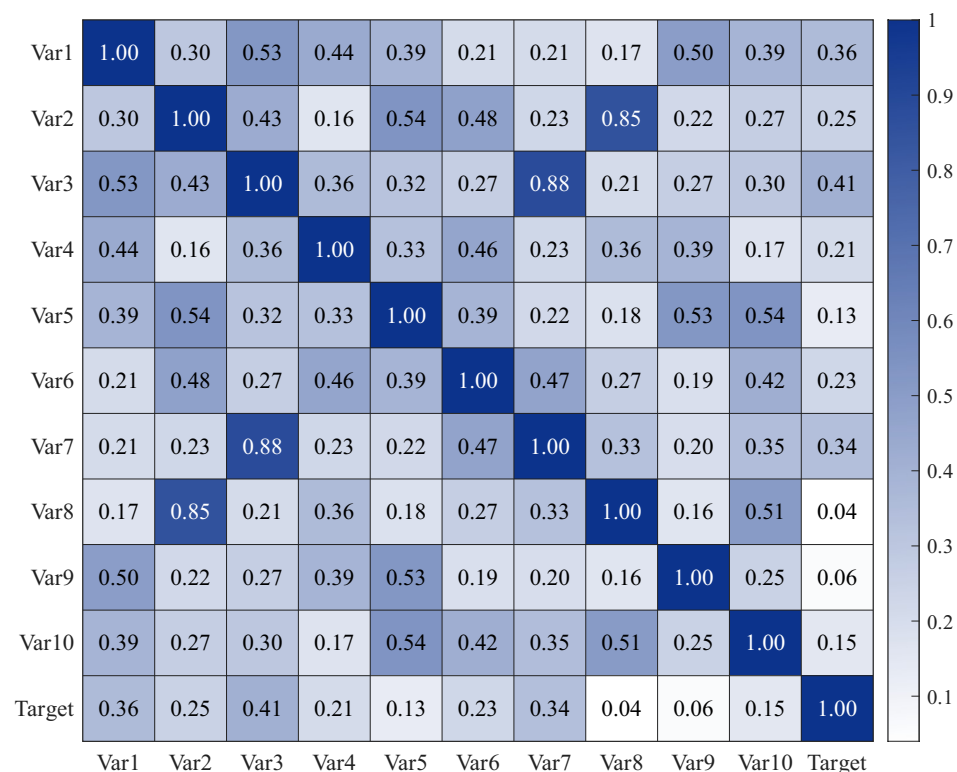
Figure 4. MIC heat map of the candidate variables and the target stack \text{NO}_x concentration.
