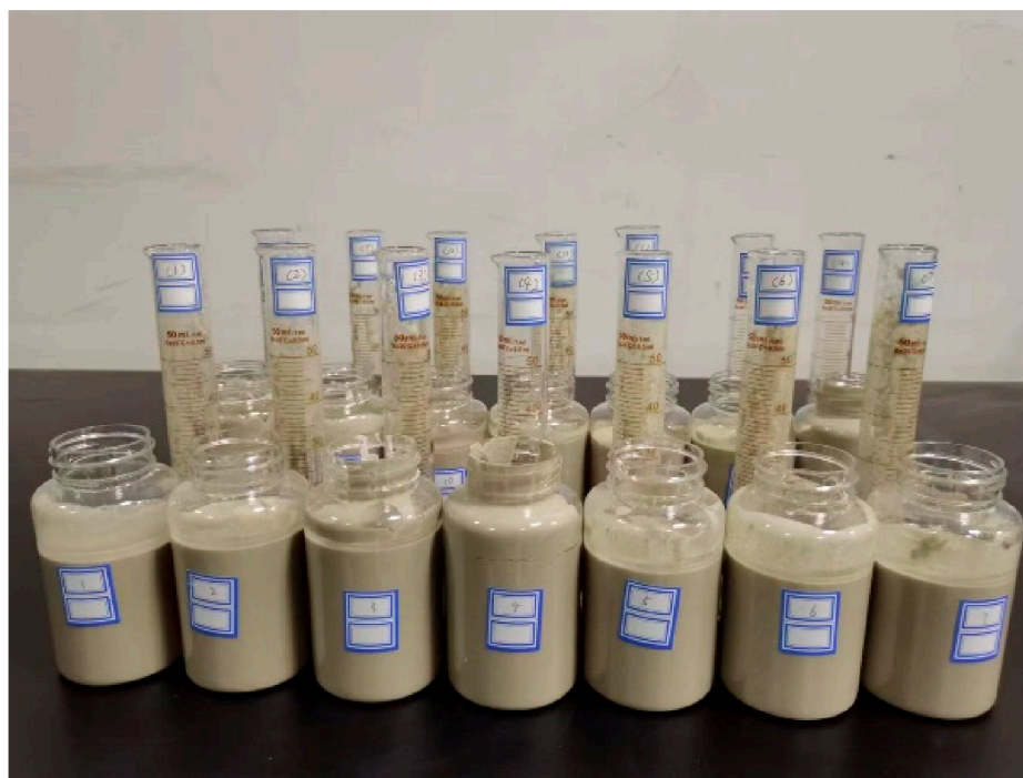
Figure 4. Bleeding rate test of BSS.
