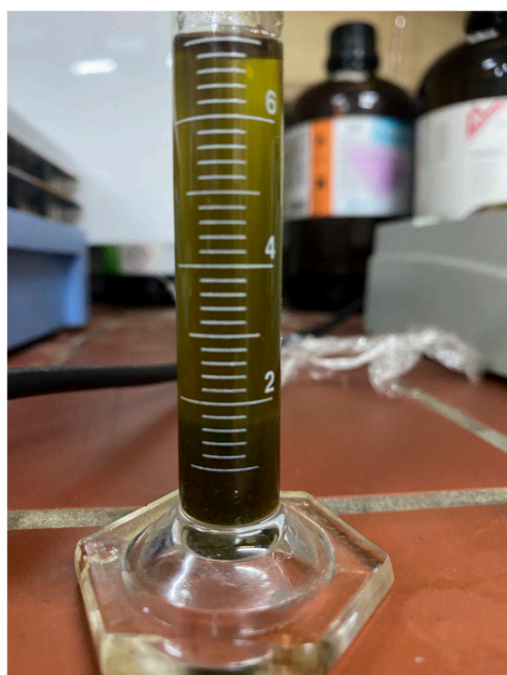
Figure 3. Volumes of the liquid extract and the solid phase (dry algae + trapped solvent) after mixing 7 mL of DMCHA with 1 g dry algae in the form of fine powder.
