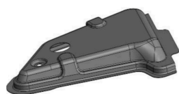
Figure 2. CAD model of car door accessory.
