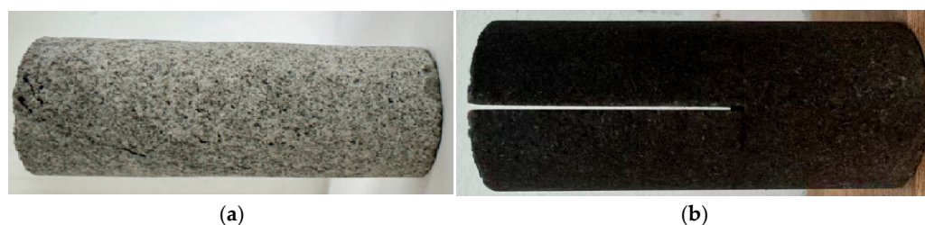
Figure 1. Photograph of the core sample from Well NC002. (a) The core sample from Well NC002, (b) The core from Well NC002 with an artificial fracture.
