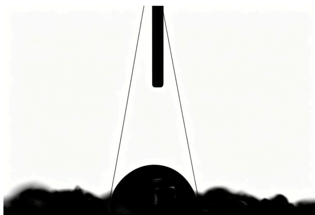
Figure 3. Static water contact angle of the PEG-grafted polyurethane sponge.
