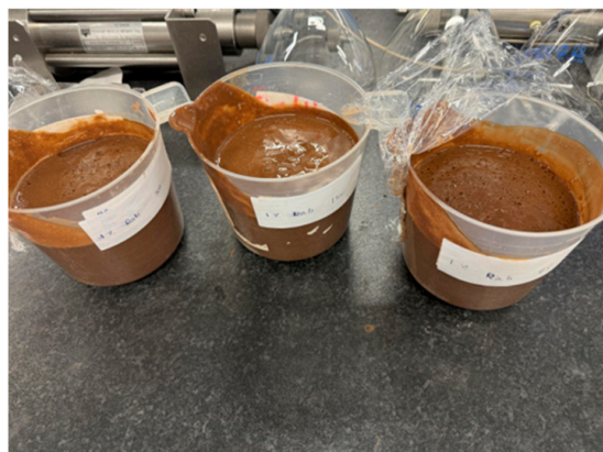
Figure 3. The prepared drilling fluid muds with various concentrations of bio-based materials.
