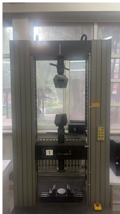
Figure 16. Electronic universal testing machine in kind and three-dimensional model drawing.
